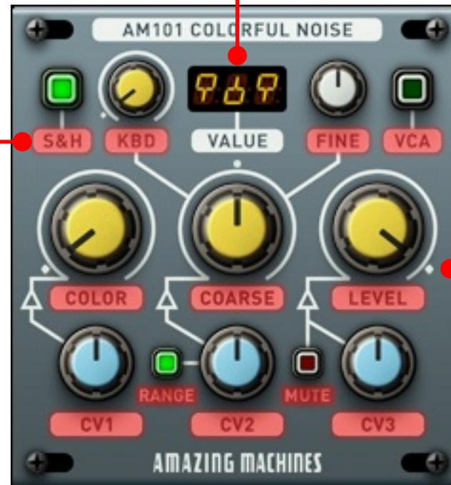
The white dots that circle around the Color, Coarse, Level and KBD knobs are Modulation Indicators, they move away from the knobs indicators depending on how the CV1, CV2, CV3 and KBD CV Inputs are set.
